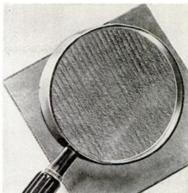
Porous, sintered plate is secret of smaller battery. It was developed by Germans before World War II
